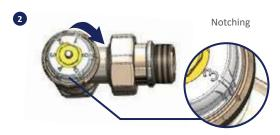
Turn the numbered handle until the number corresponding with the desired Kv (see table) is aligned with the reference notch on the valve body.
